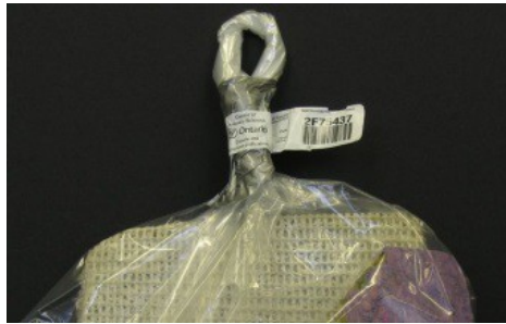
Figure 4: Speciality nylon bag with swan neck seal.
